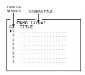
The <CAMERA TITLE> menu is composed of two screens. By rotating the JOG dial to move the cursor from its position next to the camera number to CH®, the menu will automatically scroll to the next screen.
